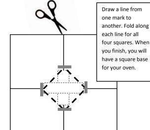
Clip panels together to form a funnel around the cook pot that will reflect light into the cooking area. Use a black pot to absorb light. Use two inverted pyrex bowls OR an oven bag as heat trap. To create a more secure surface, foil a square piece of cardboard or wood and place in the center.
